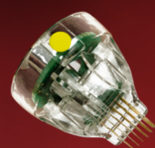
ANI-36 (36-pin) Ablative needle, insulated
